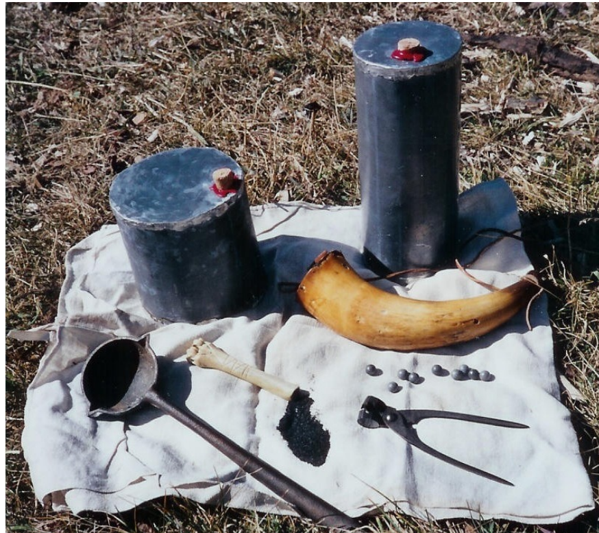
Figure 1. Lead canisters of patterns 1 and 3, an 18 th century powder horn, 0.49 caliber rifle bullets, a bullet mold, a pronghorn leg bone powder measure with a charge of powder for one bullet, and a cast iron ladle used to melt and pour lead in making bullets, all similar to artifacts probably used on the expedition. The canisters' openings are sealed with corks and sealing wax.
